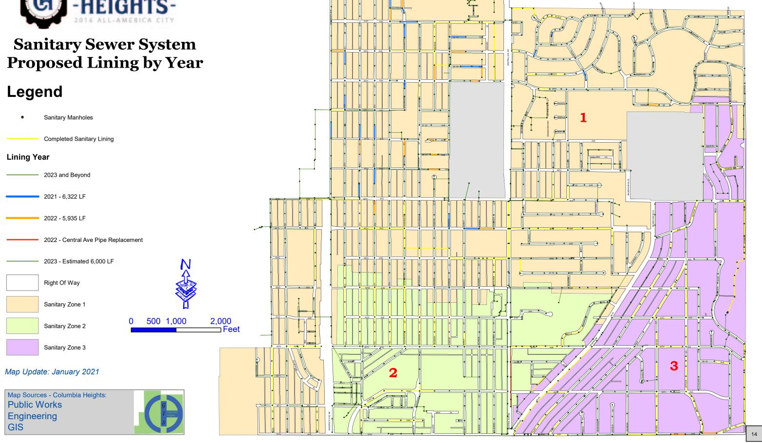
Path: Q:\gis\gisdata\Engineer\Projects\Sanitary System\SanitarySewer\_ProposedLining2021.mxd Date: 1/27/2021
